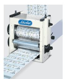
Cut & Place technology for the secure transfer of die-cut products on a continuously moving material web.
