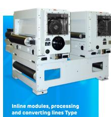
Inline modules, processing and converting lines Type SPC for production of liquid packaging blanks or rollstock. At operating speeds of up to 800 m/min and a maximum working width of 1,800 mm we do inline register-accurate creasing, perforating and die-cutting. The punching waste is removed safely.
